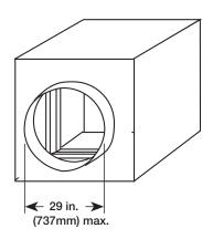
Type R transition is centered on damper frame. Dimensions are with 2 in. (50mm) offset.
